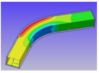
Fig 6.1 C in curve duct FD analysis of air flow
