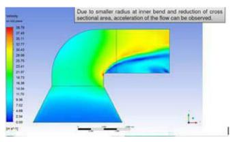
Figure 6.3 cfd analysis of air in the diffuser
